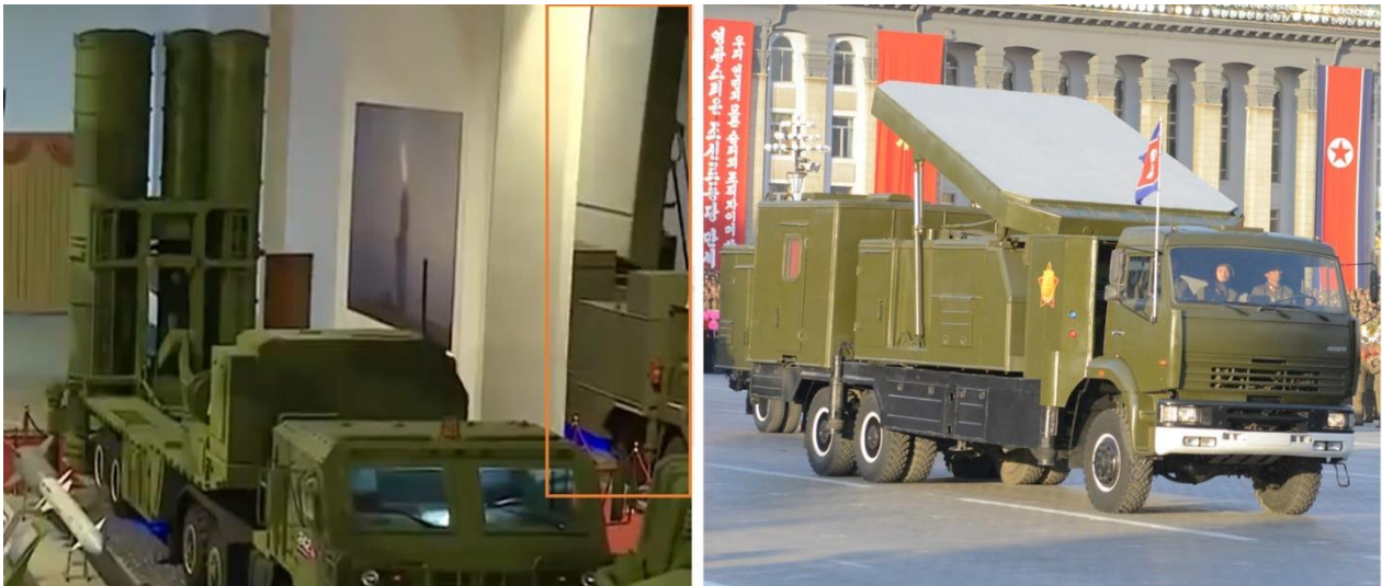
Figure 12. Partial view of a radar (left). The fire control radar of the KN-06 SAM (right). Images: KCTV (left), ONN (right)
