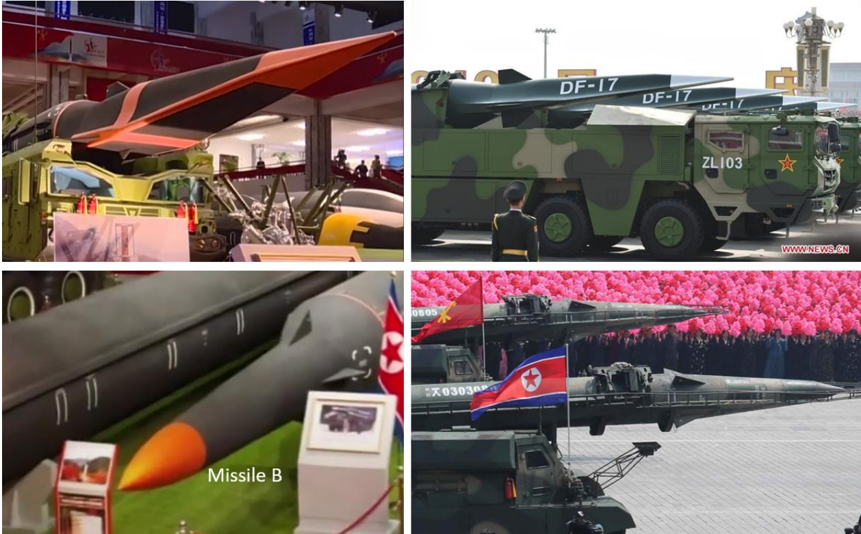
Figure 5. The warhead of the new hypersonic missile (top left) has a shape similar to that of the Chinese DF-17 (top right). The warhead of “Missile B” (bottom left) is similar to that of a DPRK precision strike variant of the SCUD missile (bottom right). The only known test of this precision strike SCUD variant was carried out on 29 May 2017. 2
