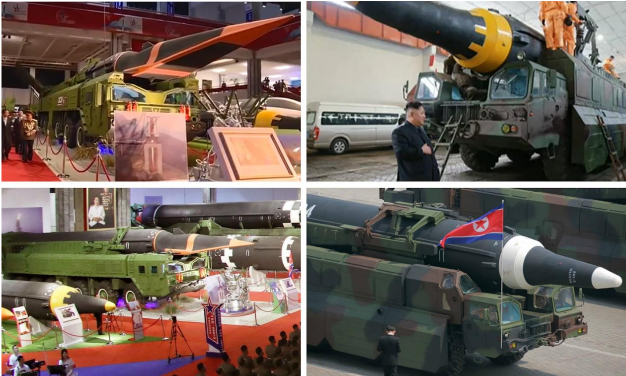
Figure 2. The new hypersonic missile in the exhibition (two photos on the left; bottom image flipped to facilitate comparison) and the Hwasong-12 IRBM (two photos on the right) are carried by the same type of TEL (in all four photos), although the TEL in the exhibition (two photos on the left) has a modified cabin, among other minor changes.
