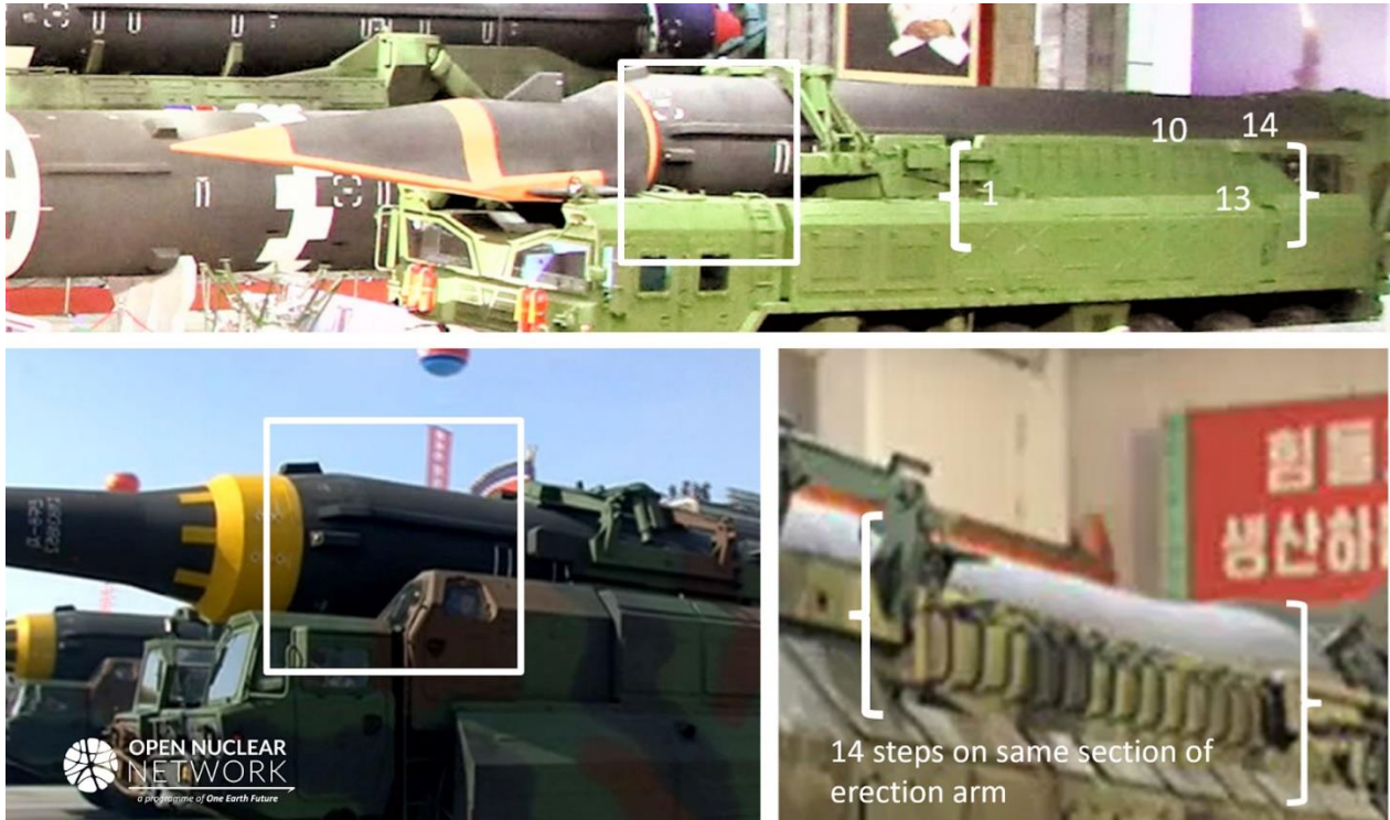
Figure 3. The number of steps on the same section of the erection arms for the new hypersonic missile (top) and the Hwasong-12 (bottom right) is the same; The sections between the upper end of the rocket stages and the upper end of the erection arms on the hypersonic missile (top) and the Hwasong-12 (bottom left) are marked in white boxes. Images: KCNA, KCTV, annotated by ONN
