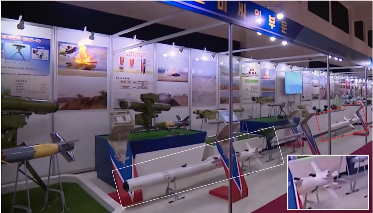
Figure 17. The missile in the white box appears to be an infra-red homing short-range AAM. The missile in the red box appears to be a radar-homing beyond-visual-range AAM. Inset photo suggests that the short-range AAM is equipped with jet vanes to improve agility. Such a design is normally seen on very advanced short range AAMs.
