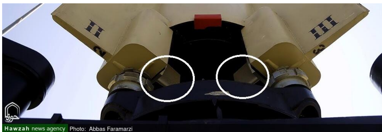
Figure 7. The Iranian Seiji solid fuel ballistic missile has bumps around its rocket nozzle. The bumps accommodate the jet vanes (in white circles), which control the attitude of the missile by directly deflecting the flame of the rocket motor. Image: Hawzah News Agency
