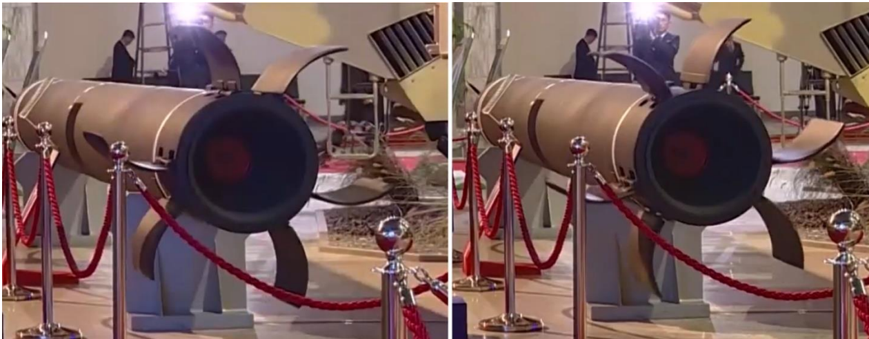
Figure 10. KCTV footage shows the rolling movement of the KN-29's tail fins on a rotating sleeve. Image: KCTV
