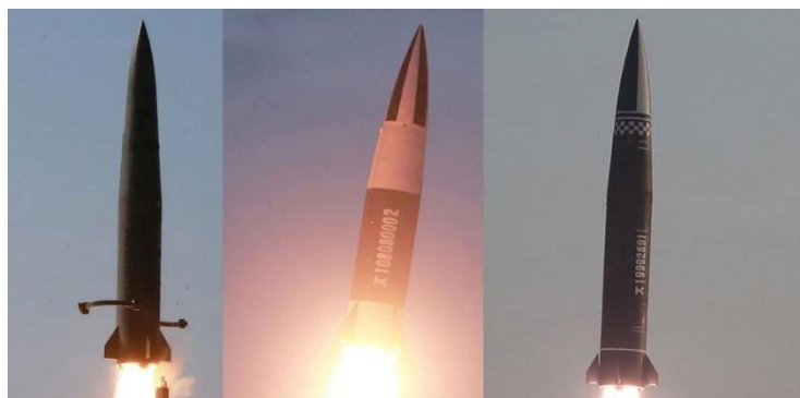
Figure 4: Left to right: KN-23, KN-24 (both test fired in 2019), new missile test fired on 25 March 2021. While the new missile appears to be a lengthened variant of the KN-23, the nose cone section is more similar to that of a KN-24. Sources: KCNA, KCTV
