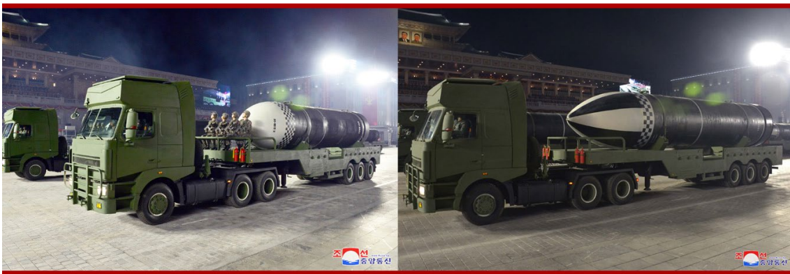
Pukguksong-4 (left) and Pukguksong-5 (right) in October 2020 and January 2021 parades, respectively. The Pukguksong-4 has a fairing similar to that of the Pukguksong-3. The Pukguksong-5 is longer than the Pukguksong-4 and also has a longer fairing.
