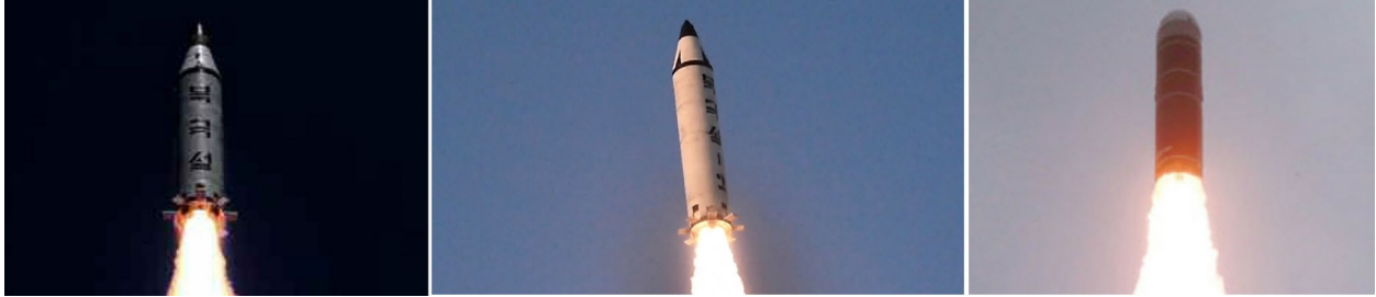
From left to right: Pukguksong-1, 2 and 3 launched in 2016, 2017 and 2019, respectively. The Pukguksong-1 and Pukguksong-2 have eight grid fins. The Pukguksong-3 has a rounded fairing presumably to improve underwater stability and has no visible grid fins.
