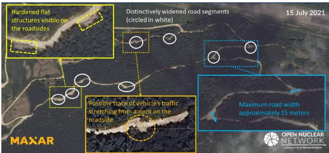
Figure 7. Widened segments along the improved mountain roads on Mount Paegyang. Image: © 2021 Maxar Technologies. All Rights Reserved. Reprinted by permission.
