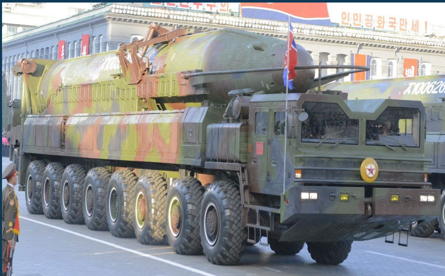
Hwasong-13 Mod 2 on a WS51200 truck in a parade on 10 October 2015. Mod 2 is a two-stage design. Source: ONN
