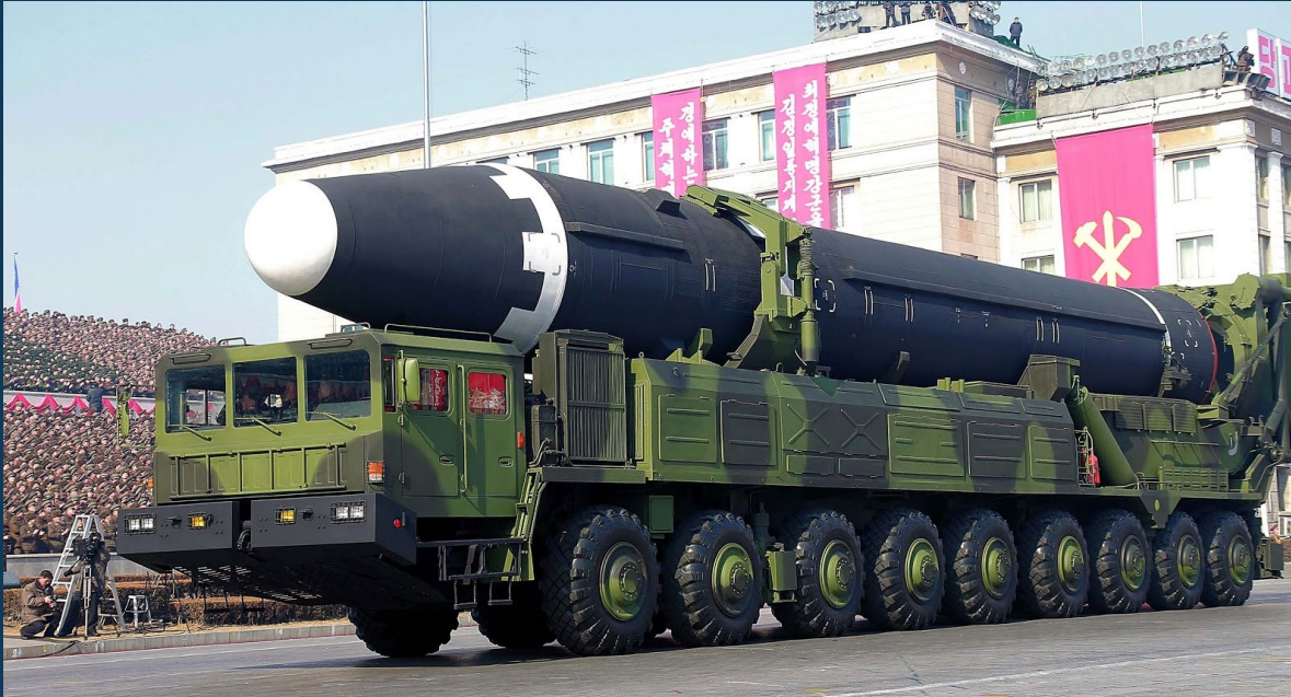
Hwasong-15 shown on a 9-axis modification of the WS51200 on 8 February 2018
