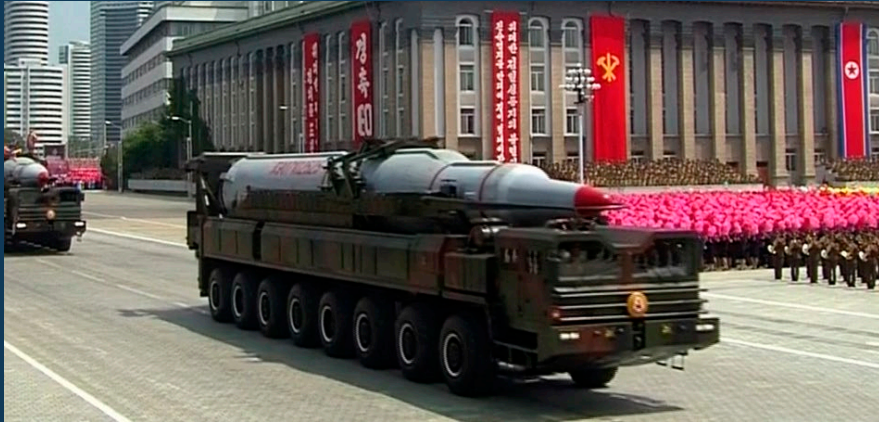
Hwasong-13 Mod 1 on a WS51200 truck shown at a parade on 15 April 2012. Mod 1 is a three-stage, liquid propellant design. Source: KCTV
