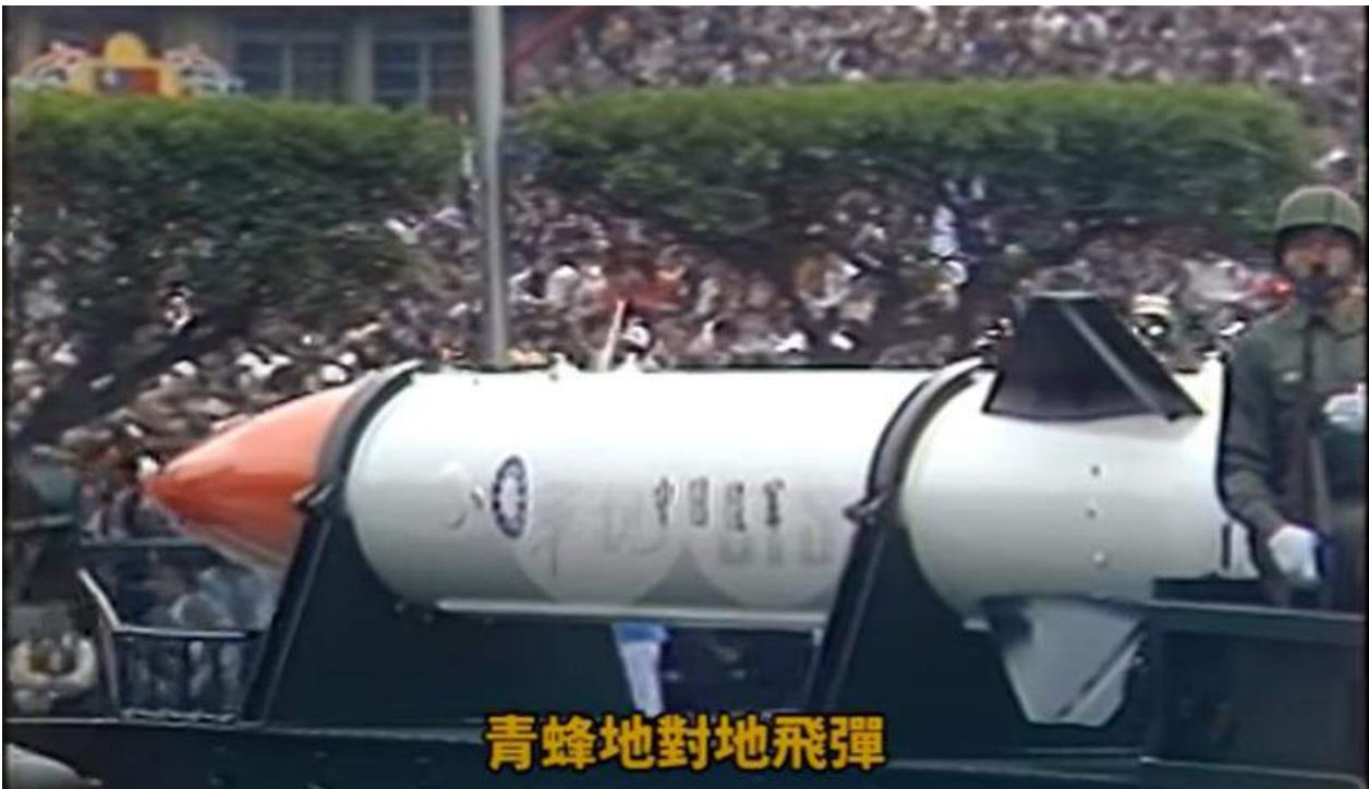
Figure 1. The Chieng Feng solid propellant, short-range ballistic missile. Image: CTS News 6
