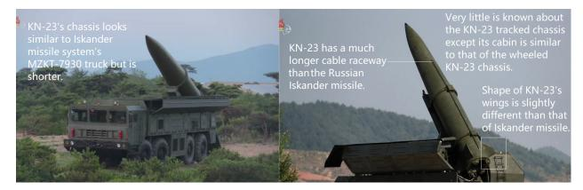
In its first two launches four KN-23 missiles were fired along with other long-range artillery projectiles as part of joint strike drills. All KN-23 missiles launched were painted in an army green colour scheme. KN-23 has both tracked and wheeled chassis. The overall appearance of the wheeled chassis shares some similarities to the Iskander missile system's MZKT-7930 truck. Image: KCTV, annotations by authors.
