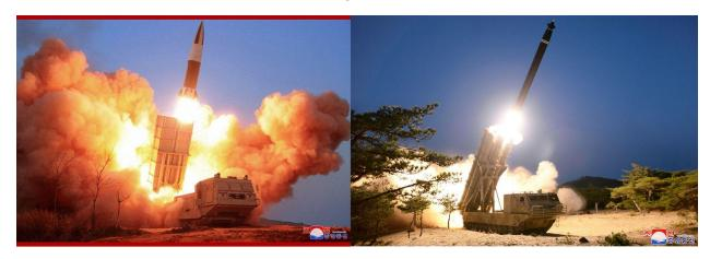
The KN-24 SRBM's tracked chassis is similar to that of the KN-25 "super large calibre" MRL (right). Both have driving wheels located in the front but the KN-24 has six road wheels on each side, while the KN-25 has 10 road wheels. All KN-24 missiles launched were painted with a distinguishable testing paint that serves tracking and measurement purposes. Image: KCNA.
