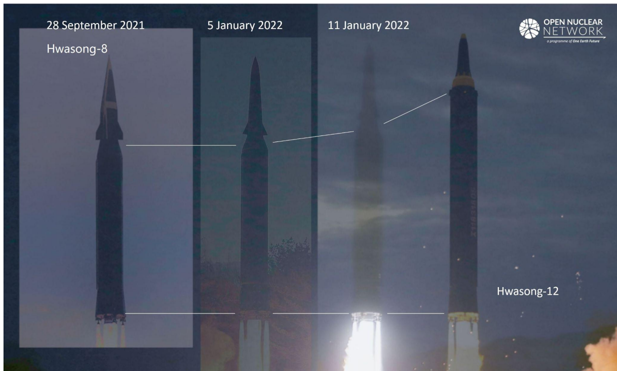
Figure 2. White lines mark the length of the rocket stages. Images: KCNA
