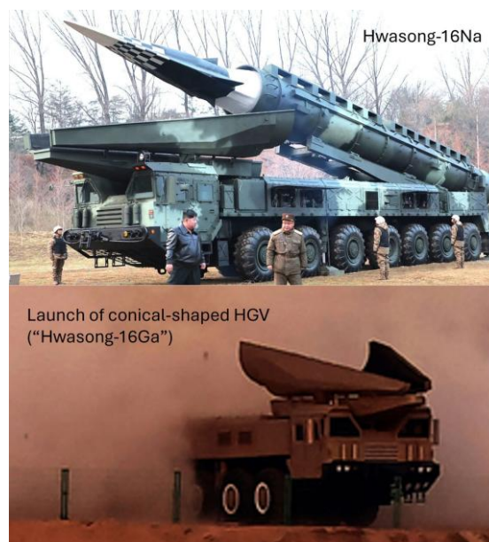
Figure 7. The TEL’s cabin and the protective cover for the Hwasong-16Na (Top) appear to be identical or similar to that of the “Hwasong-16Ga” (Bottom).
