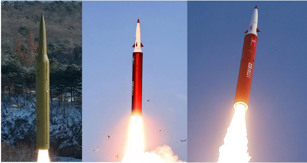
Figure 6. Except for the paint scheme, the hypersonic missile (referred to as “Hwasong-16Ga” for the purpose of the article) launched on 3 October (Middle, Right) appears to be identical or very similar to the one launched in January 2024 (Left).
