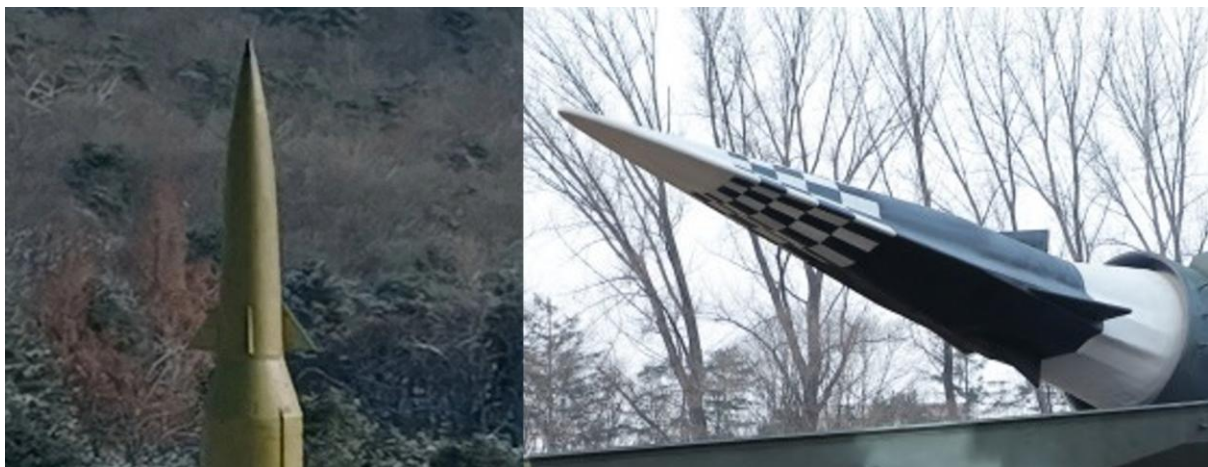
Figure 4. The conical-shaped HGV (left, referred to as “Hwasong-16Ga” for the purpose of this article) has a much simpler aerodynamic layout than the wedge-shaped Hwasong-16Na. Images: KCNA
