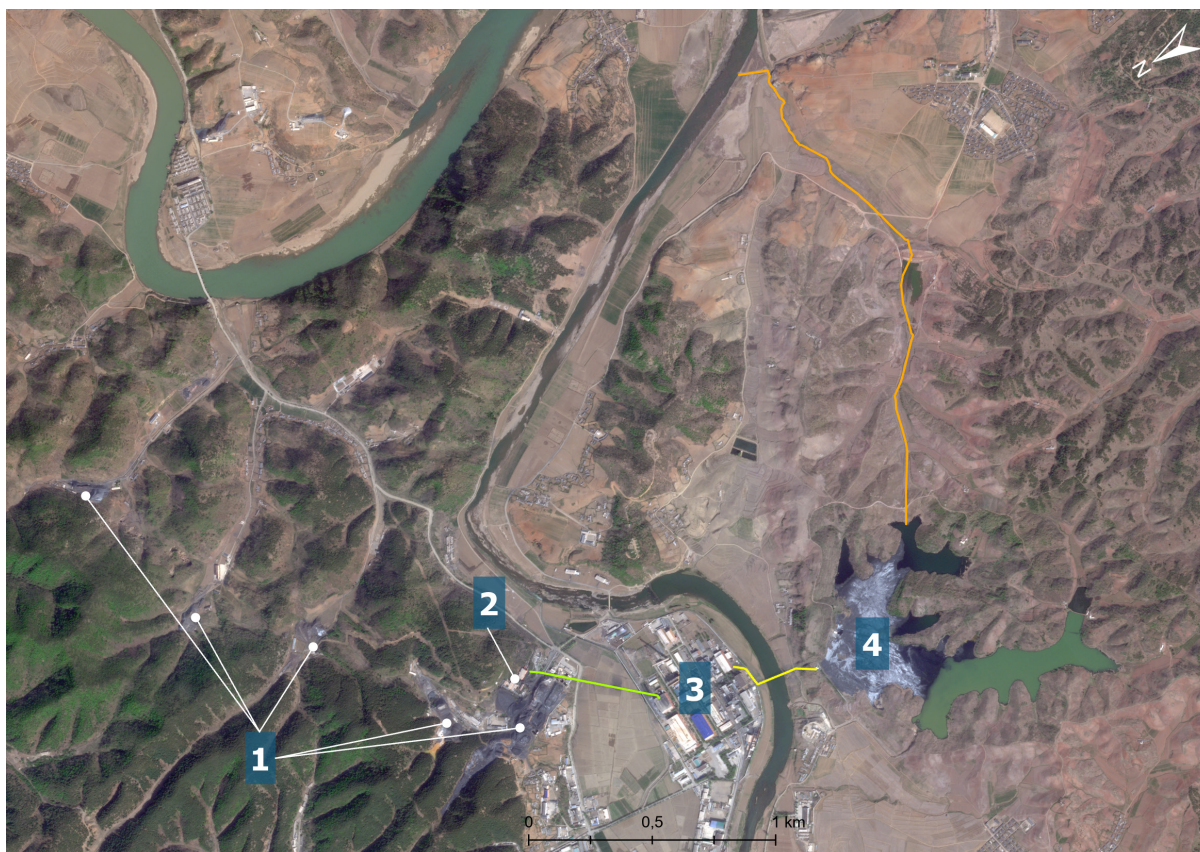
Figure 4: Pyongsan complex. 1 – mines; 2 – crushing and grinding mill; 3 – Concentration Plant; 4 – tailings pond. Green line – pipeline from milling to the Plant; yellow – pipeline to the tailings pond; orange – wastewater path to the river. 38.318 N, 126.434 E. 19 April 2026. Image: © 2026 Planet
