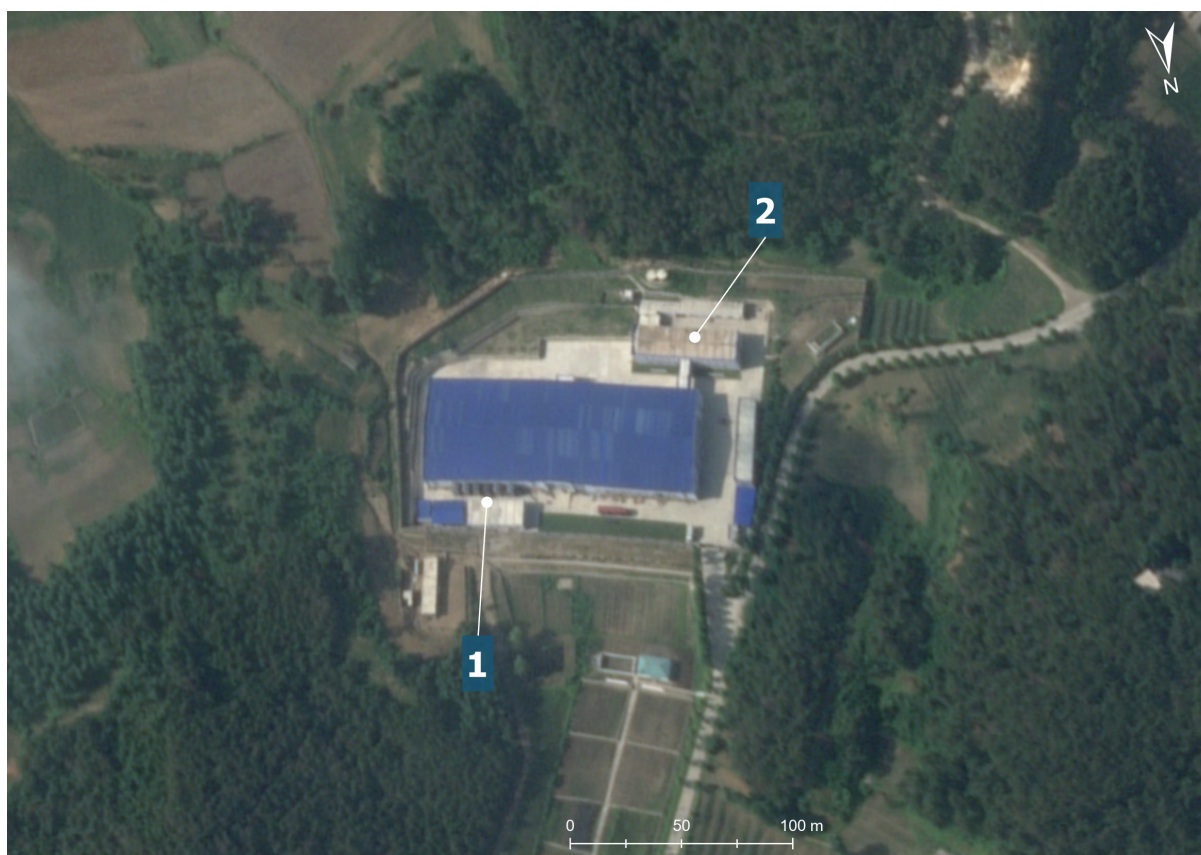
Figure 7: New enrichment building at Yongbyon. 1 – probable ventilation stack; 2 – support building. 39.785 N, 125.759 E. 27 June 2026. Image: © 2026 Planet
