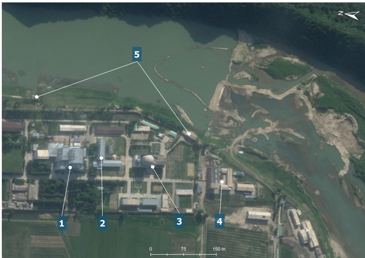
Figure 9: Reactors area. 1 – 5 MWe reactor; 2 – spent-fuel storage; 3 – ELWR; 4 – ELWR support facility; 5 – water pump houses. 39.796 N, 125.755 E. 27 June 2026. Image: © 2026 Planet
