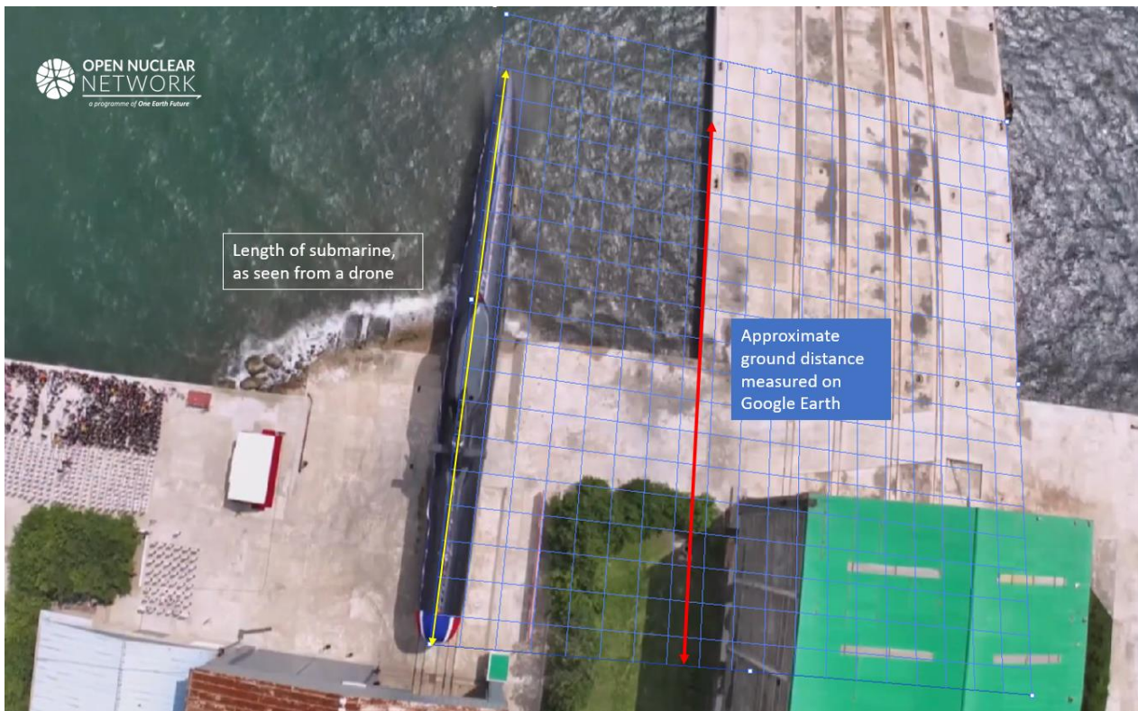
Figure 4. A grid is established 28 to eliminate errors caused by perspectives and to virtually move the submarine to the same vertical plane where a measurable reference exists, which enables the ground distance covered by the submarine (the actual length) to be measured on Google Earth.
