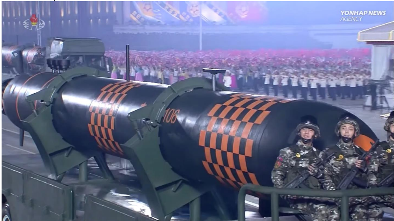
Figure 2. Underwater nuclear attack drones at the 27 July parade. As the DPRK navy is not known to have super-large torpedo tubes, it is possible that this drone is either directly launched from shore or released by surface vessels.
