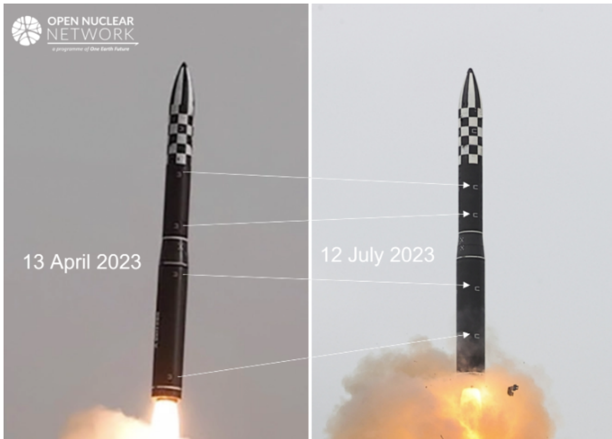
Figure 2. Although there are few visual differences between the Hwasong-18s launched in April and July, different positions of the markings suggest that supporting structures inside the launch tube might have been adjusted. Images: KCNA , KCNA
