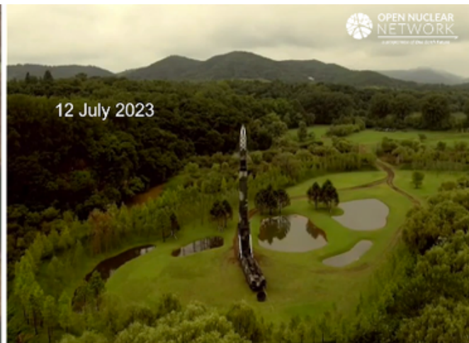
Figure 3. Left: Flame and smoke produced by a gas generator, designed to eject the missile out of its tube, emanated from the bottom of the launch tube, suggesting a possible leakage during the first test on 13 April 2023. Right: No indication of leakage during the 12 July 2023 test. Images: KCTV , KCTV
