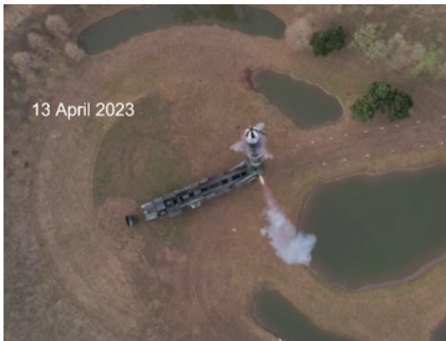
Figure 3. Left: Flame and smoke produced by a gas generator, designed to eject the missile out of its tube, emanated from the bottom of the launch tube, suggesting a possible leakage during the first test on 13 April 2023. Right: No indication of leakage during the 12 July 2023 test. Images: KCTV , KCTV
