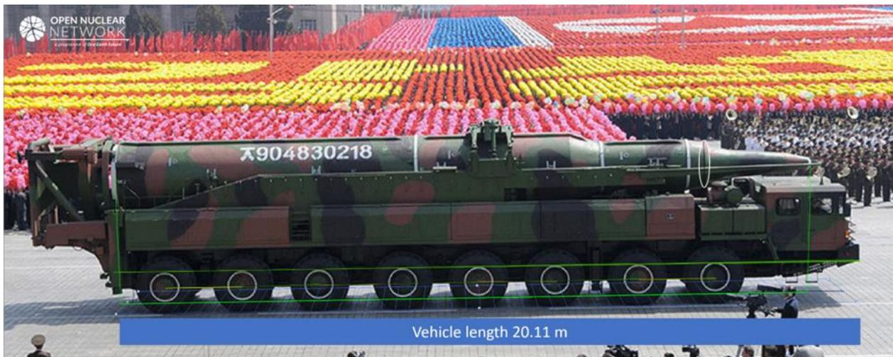
Figure 7. Using stated length of WS51200 truck as reference, approximate length of the missile and base diameter of its re-entry vehicle could be measured.
