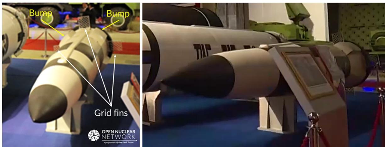
*Figure 1. The small SLBM that made its public debut at the exhibition on 12 October (left and right). The grid fins installed between the bumps are meant to increase the stability and possibly control the attitude of the missile during the ejection process. Images: KCNA, KCTV, annotated by ONN*
