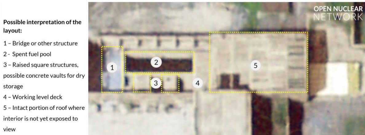
Figure 5. One possible interpretation of the interior layout of the building. Image © 2021 Planet Labs Inc. All Rights Reserved. Reprinted by permission.
