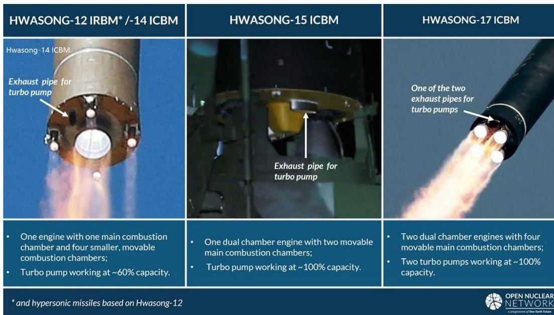
Figure 3. Common engine technologies shared by the DPRK’s new generation of liquid-propellant ballistic missiles. Images: KCNA, annotated by ONN
