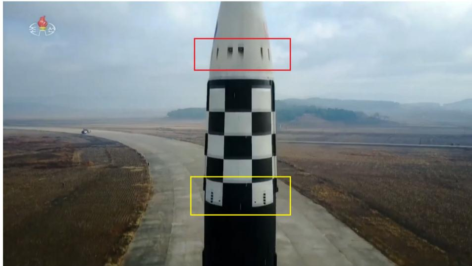
Figure 2. Inside red box: fairing removal rockets; Inside yellow box: possible nozzles of eight small rockets whose role may be to help ensure a smooth separation of the warhead after second stage burnout. Image: KCTV
