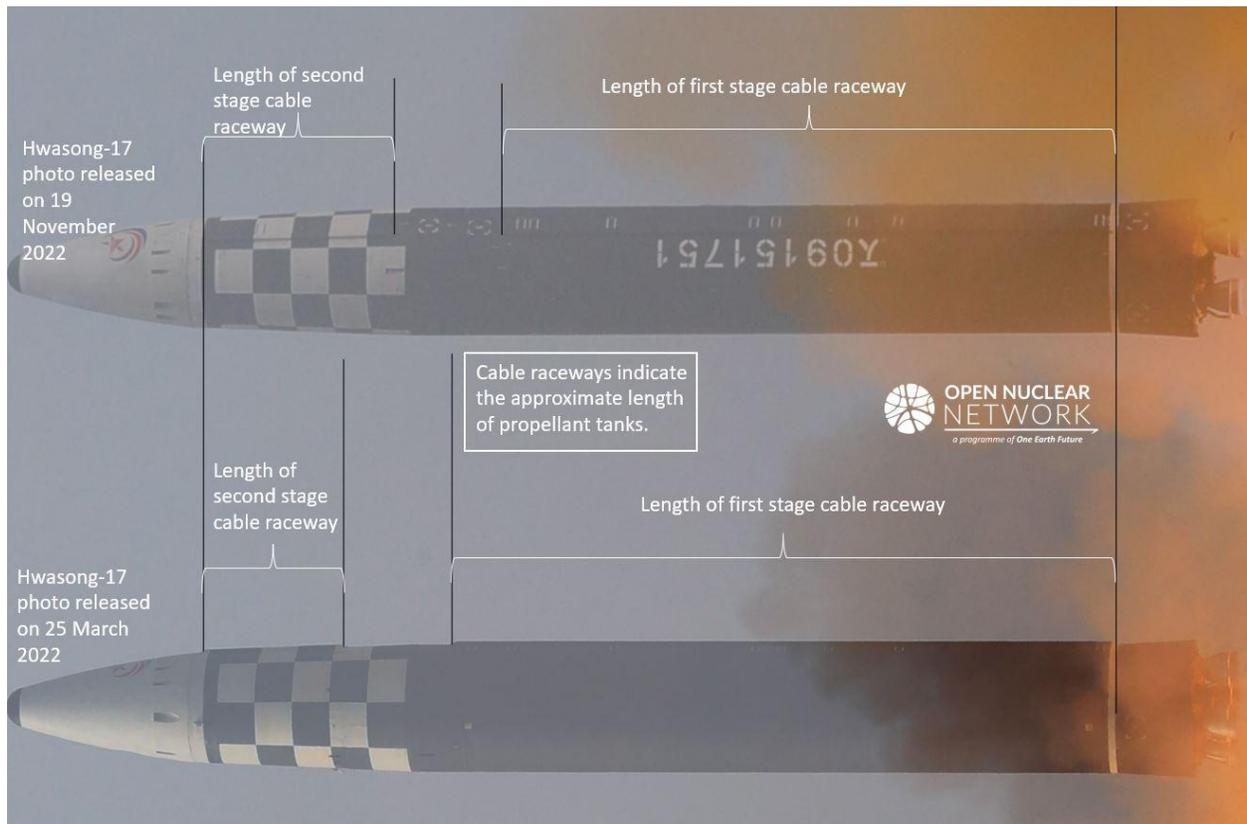
Figure 1. Differences between the two Hwasong-17 prototypes. Images: KCNA
