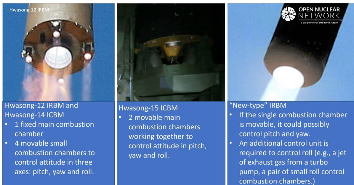
Figure 1. Comparison of the propulsion units between existing Hwasong strategic missiles and the "new-type" IRBM. Images: sogwang media corporation, KCNA, KCNA/Reuters[2]
