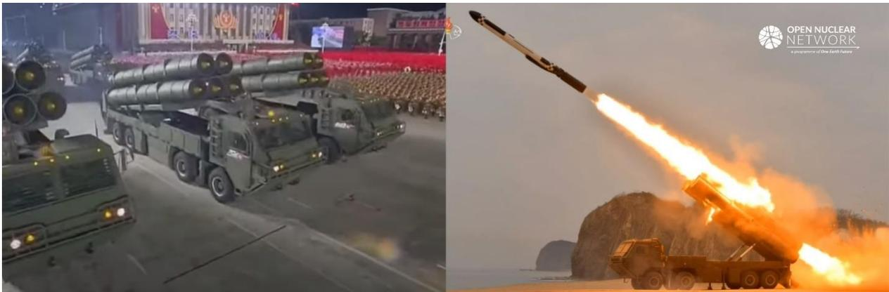
Figure 8. Left: Parade vehicles carry models of five model rounds of “super-large calibre multiple rocket launchers (MRLs)” during the October 2020 parade. Right: Same launcher with parade configurations fires a land-attack cruise missile from one of its five launch canisters. Images: KCTV [26]
