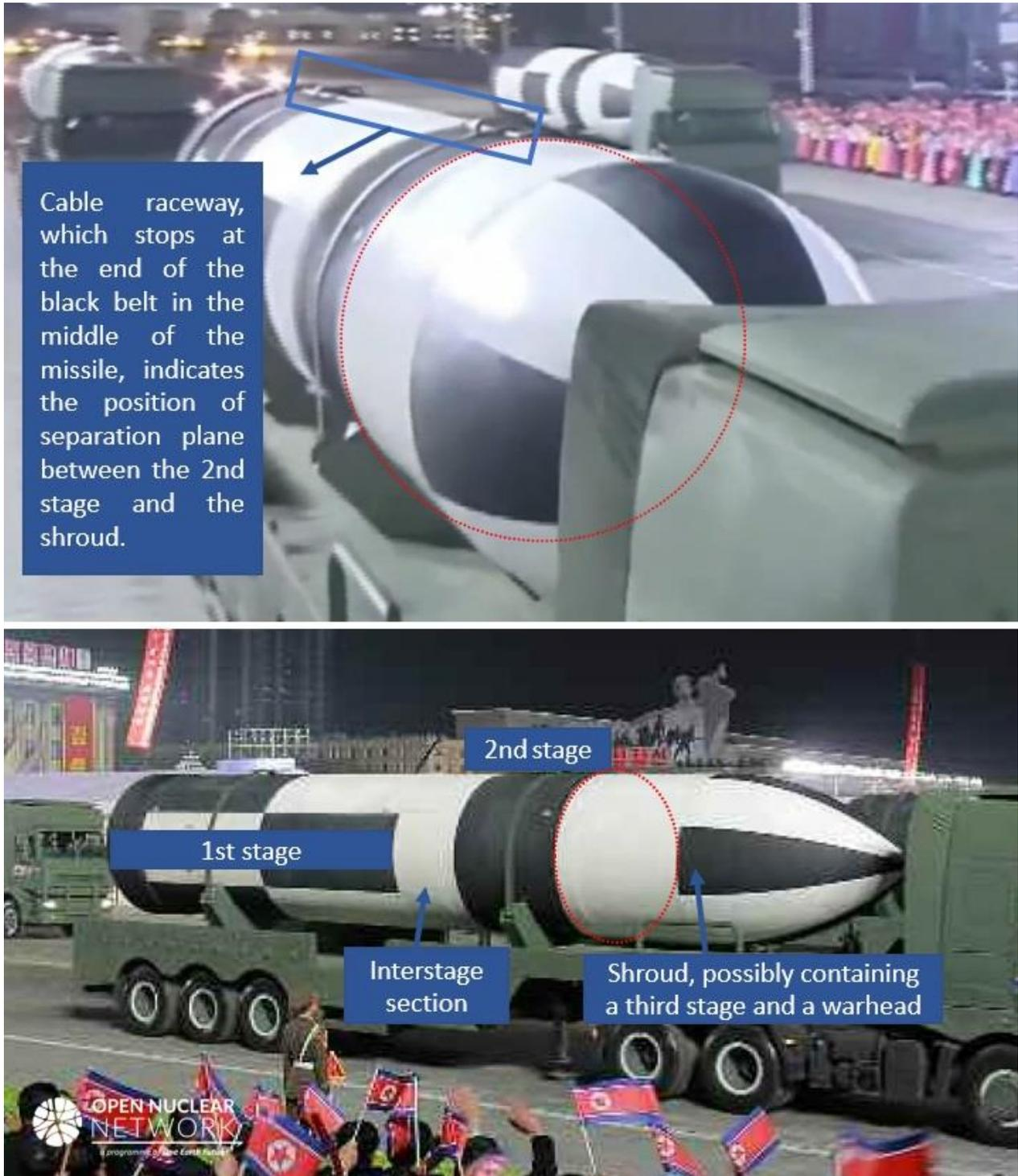
Figure 5. The cable raceway is indicative of the length of each stage of the unnamed SLBM because the cables could not be placed inside the propellant. The shroud seems to have enough length and volume to accommodate a third stage and the warhead.
