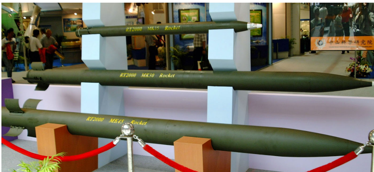
Picture shows Taiwan's MK15, MK30 and MK45 MRL rounds with both folded and unfolded wrap-around fins.
