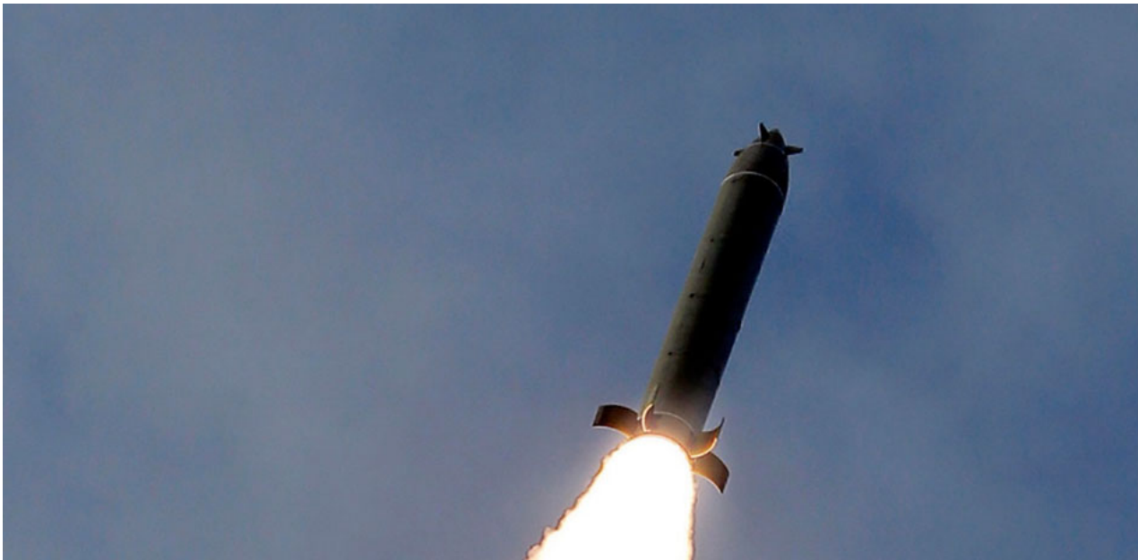
North Korea's "super large calibre MRL" rocket, codenamed KN-25, has six wrap-around fins. Every two of the fins form a pair of brackets. Photo: KCTV
