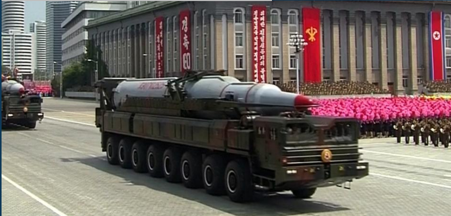
Hwasong-13 Mod 1 on a WS51200 truck shown at a parade on 15 April 2012. Mod 1 is a three-stage, liquid propellant design. Image: KCTV
